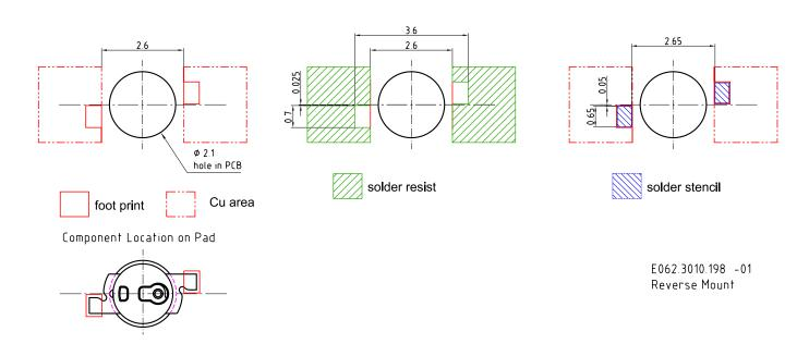
For superior solder joint connectivity results we recommend soldering under standard nitrogen atmosphere. Package not suitable for ultra sonic cleaning.
